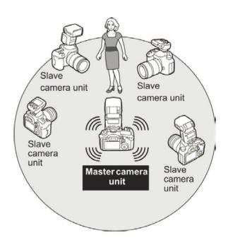
Among cameras with a 430EX III-RT attached, it is possible to simultaneously release the shutters of slave and master cameras with their sync function.
